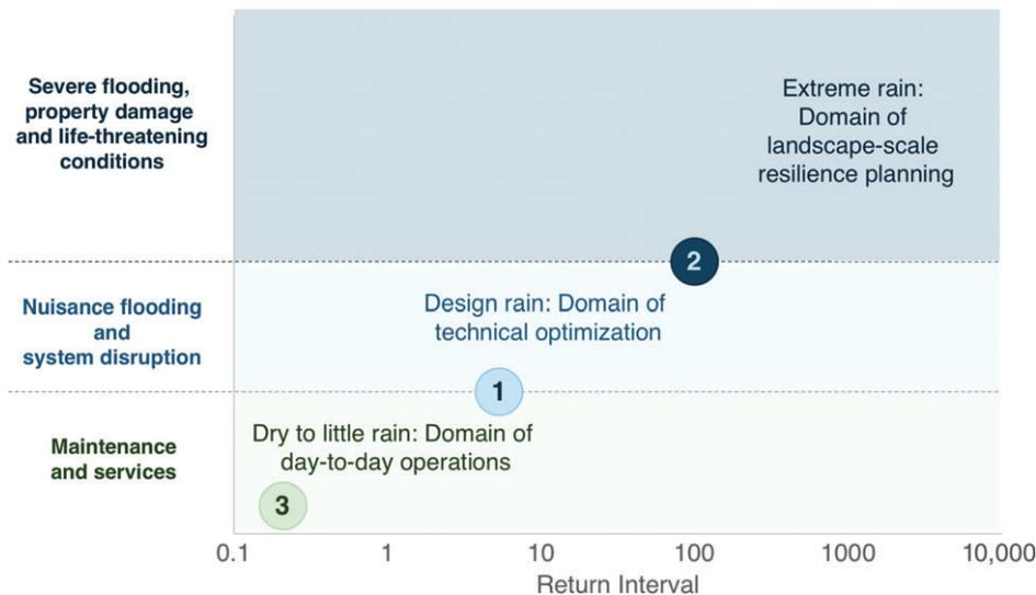
**FIGURE 6** Three points approach scheme for pluvial flood management. The horizontal axis represents the rain event return interval and the vertical axis represents the magnitude of impacts. Both axes are on a logarithmic scale. The three “points” represent thresholds for each management domain. (Modified from Fratini et al. (2012))
