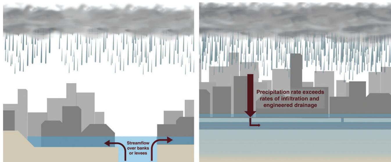
**FIGURE 1** Fluvial (left) versus pluvial (right) flooding. Fluvial flooding occurs when water routed by streams, rivers or equivalent water bodies overflows its banks, inundating the adjacent floodplain area. Pluvial flooding occurs when precipitation rates exceed the infiltration capacity of soils and the drainage capacity of stormwater infrastructure, resulting in ponding and overland flow
