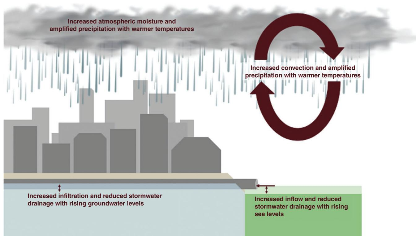
**FIGURE 5** Potential mechanisms by which climate change can increase pluvial flood hazard in cities. Climate change can directly increase the frequency, spatial extent and magnitude of intense rain, which can result in exceedance of designed drainage capacity
